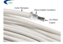
ELTEC SILICONE RUBBER INSULATED CABLES with FIBER GLASS BRAID are used for high temp. applications. It has an excellent die electric properties when burnt and in addition these cables are flame retardant and self extinguishing. These cables are also resistant to fungus, UV radiations, corona discharge, acids and manganese.
