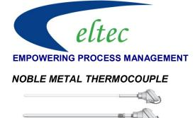
Noble Metal Thermocouple usually designed for extremely high temperature applications mostly above 1000 °C and hence uses High Alumina Content Ceramic tubes as outer protection for thermocouple junction. They have good resistance to thermal shock but poor resistance to mechanical shock; they should be mounted vertically.
