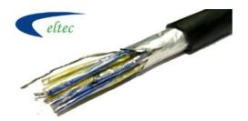
In an industrial environment of induced voltage and electrical noise, PVC Insulated twisted overall shielded thermocouple pairs is an ideal selection. Twisted pairs & aluminum Mylar shield provides protection against cross talk, static & magnetic noise in thermocouple circuits.
