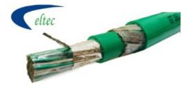
Armored Thermocouple Extension Wires are used for underground applications as GI wire armoring gives strong mechanical protection. Twisted pairs & aluminum Mylar shield provides protection against cross talk, static & magnetic noise in thermocouple circuits.
